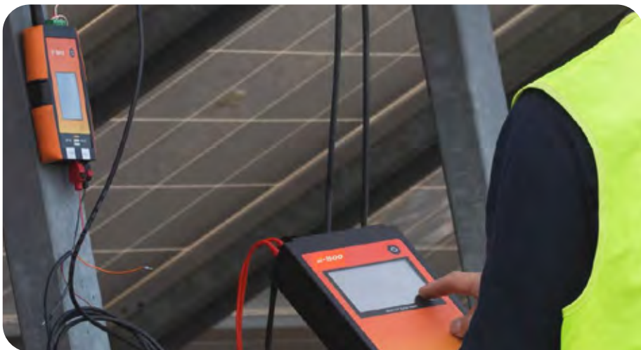
Figure 3: I-V curve measurement screen, E-1500 curve tracer, bifacial module.
