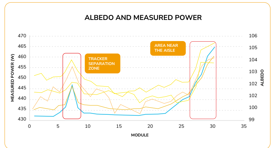
Figure 1: Impact of rear cell placement on albedo measurement. The blue line corresponds to the albedo.
